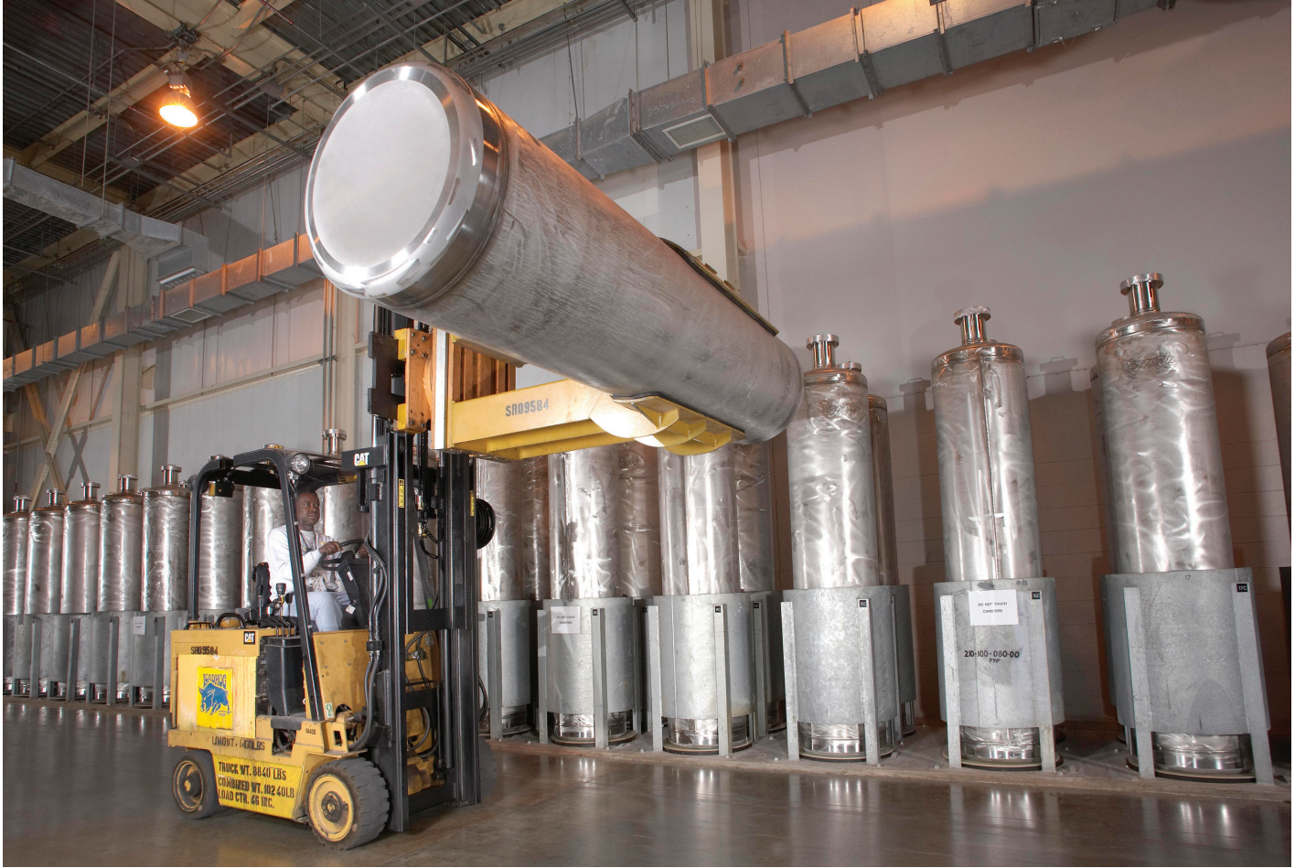
In the can-in-canister approach, canisters are filled with vitrified highly radioactive waste, and stored in the Defense Waste Processing Facility.
