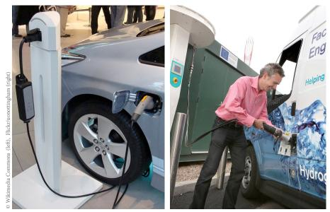
Neither plug-in (left) nor hydrogen (right) EV technologies use oil and both reduce global warming emissions compared with their gasoline and diesel counterparts.
