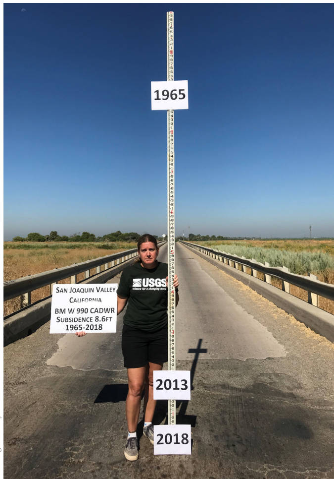
Between 1965 and 2018, some parts of the San Joaquin Valley sank 8.6 feet, a phenomenon known as land subsidence that is exacerbated by aggressive overpumping of groundwater. Because the land sinks unevenly, this can have devastating impacts on infrastructure such as roads.
