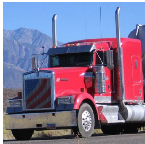
Typical classic styled truck with long nose, flat bumper, low-roof, and exposed air cleaners, exhaust stacks, and fuel tanks.
