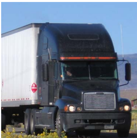
Aerodynamic styled truck with low profile front, aerodynamic bumper, full-height roof fairing, hidden exhaust stacks, and fuel tank side fairings.
