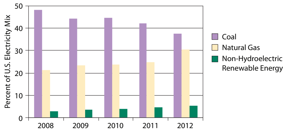
Coal's share of U.S. electricity generation shrank from 48 percent in 2008 to 37 percent in 2012, while natural gas grew to more than 30 percent and non-hydro renewables to 5.4 percent (EIA 2013b).
