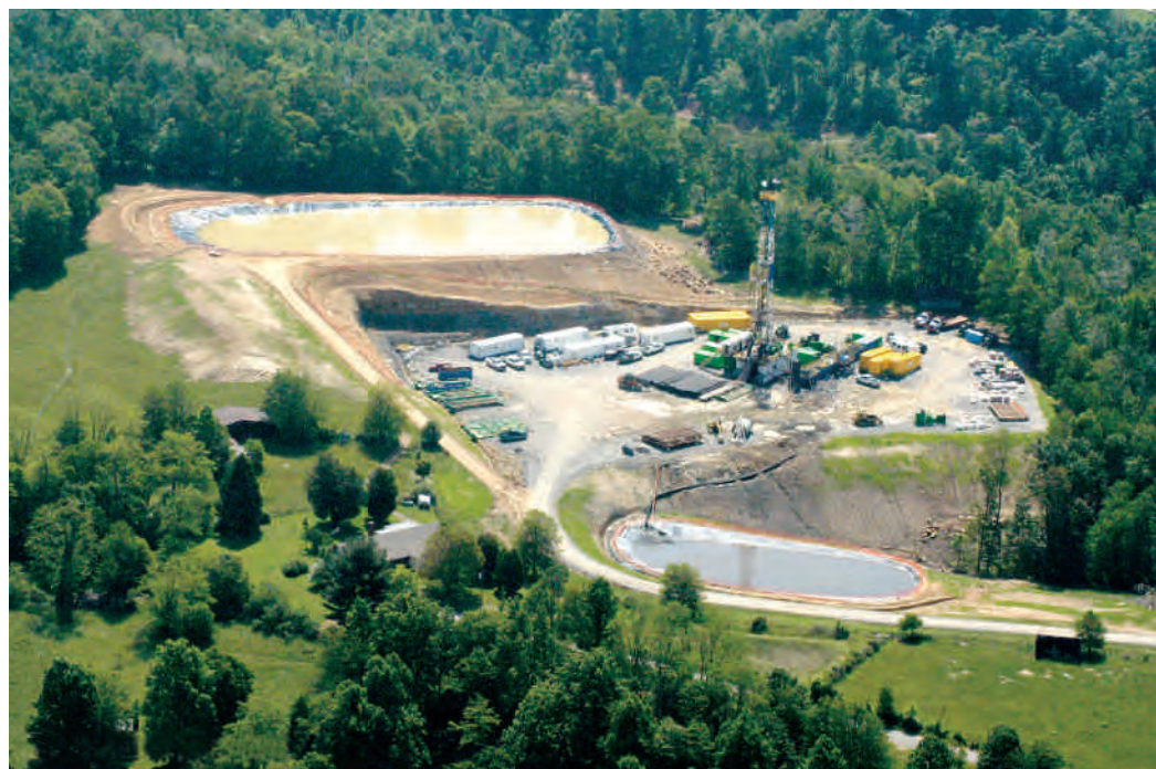
A well site in Upshur County, West Virginia—sitting atop the extensive Marcellus Shale Formation—shows a hydraulic fracturing operation. The drilling and extraction of natural gas, and its distribution in pipelines, also results in the leakage of methane—a more potent heat-trapping gas than carbon dioxide.
