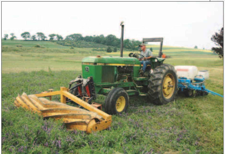
This roller-crimper tractor attachment is designed for organic no-till farming. Here, it is crushing a cover crop called hairy vetch into mulch, with little soil disturbance. This practice keeps most carbon in the ground, while the compressed crop suppresses weeds, contributes nitrogen and moisture to the soil, and creates habitat for insects beneficial to the corn that is simultaneously being planted.
