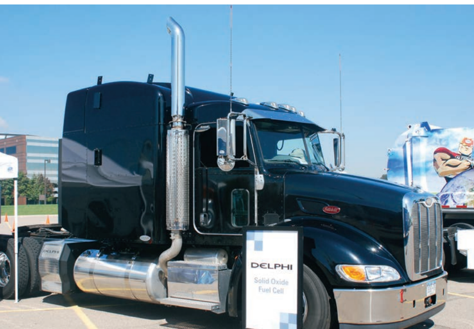
A fuel cell auxiliary power unit (located to the left of the diesel tank and in front of the rear wheels in this photo), eliminates exhaust emissions while delivering power to the cab during rest periods.
